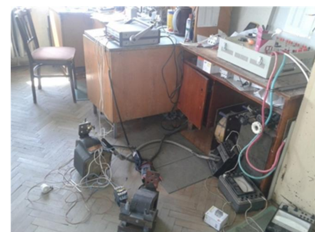
Fig.5. Carrying out the laboratory experiments with the protection system against overvoltages and the current transformer type TLM-10 (TJIM-10)
