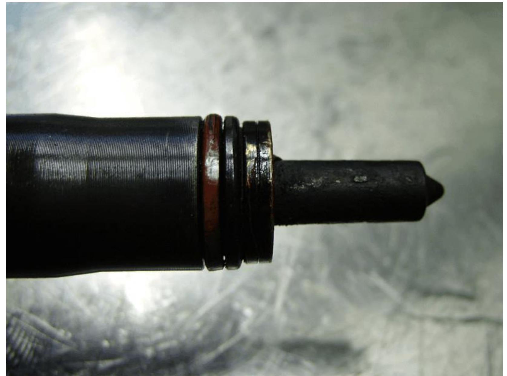
Fig. 3. Example of wear of the injector tip. [2]
