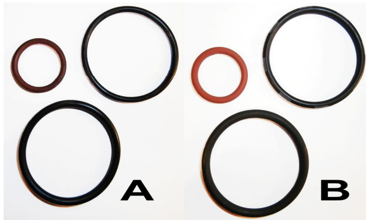
Fig. 3. Photos of external unit injector seals; A) old, B) new.
