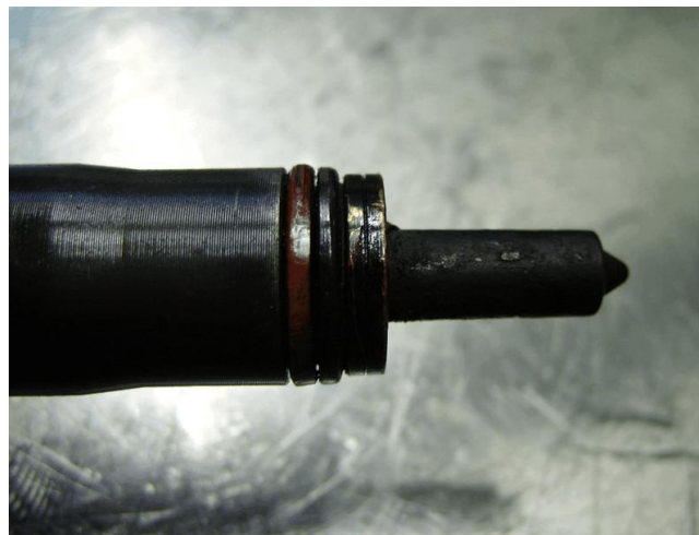
Fig. 4. Example of wear of the injector tip [4]
