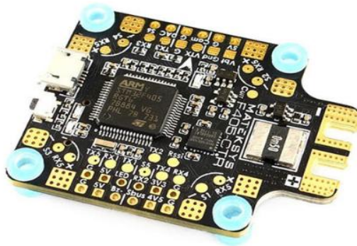
Fig.1. Matek Systems F405-CTR Controller
